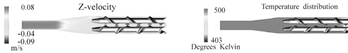
Figure 9. Axial, z-velocity, and temperature distributions at the die and pressurization section of the universal twin-screw extruder for 100 rpm, 180°C, and 72.3 lb/h.
